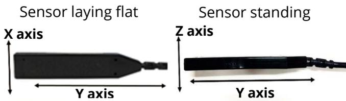
Note: The Y axis is always the direction of the cable.
