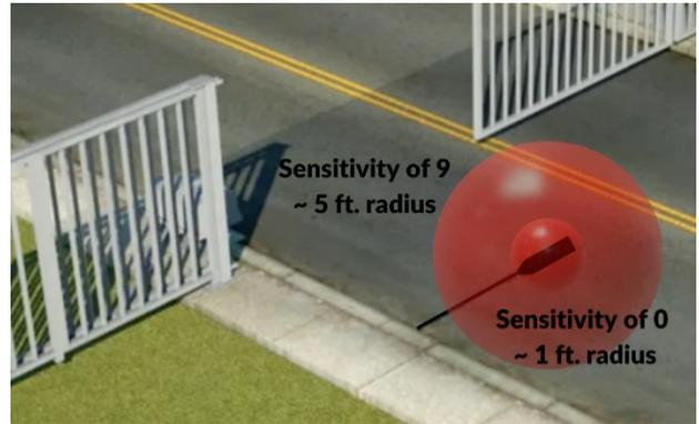
6. After the sensor is working correctly, cut the pavement according to the instructions starting below. **Use a hard sealant, such as epoxy, around the sensor. The sealant fill should not extend above the roadway.** Incorrect fill allows vehicle weight to press on and move the sensor in the concrete, which will cause the sensor to go into detection. **Press the RESET button on the CS303-C-1 once the sensor is in place.**
