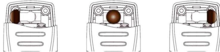
Units should be placed a minimum of 12 – 16 inches from the floor. Across from and lenses facing each other. The receiver red detect LED will be on when the beam is broken or not aligned.
